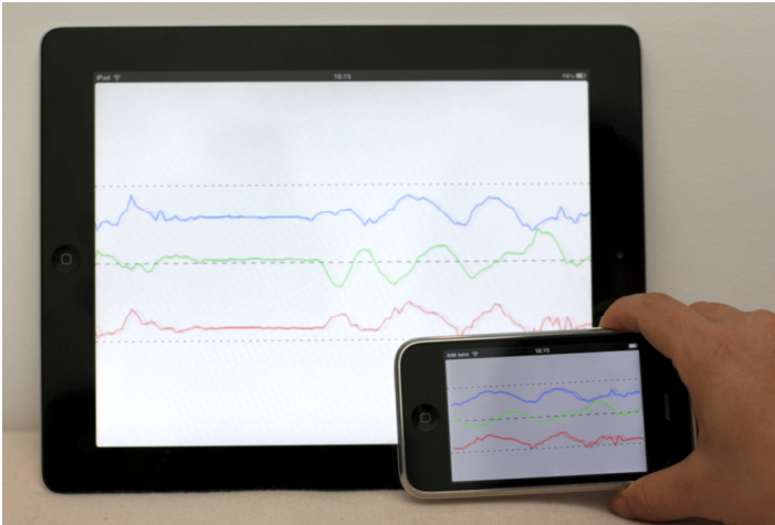
Figure 1. The inertial sensor data captured by the smartphone is streamed to the tablet computer and visualized. Here, the accelerometer sensor data is shown. The three dotted lines mark an acceleration of -1g , 0g , and 1g . (See full color version at www.performance-science.org .)
