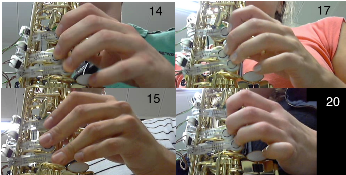
Figure 1. Screen shots of four participants, with fingerings for g' on alto saxophone. Depending on their playing technique, they cover the force sensors (left) or only touch a part of it (right). (See full color version at www.performance-science.org .)
