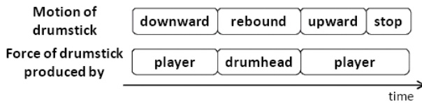
Figure 1. Motion of drumstick and force of drumstick for a single stroke.
